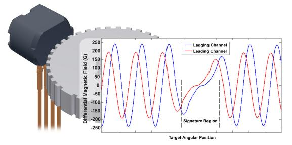
Figure 1: The use of an integrated magnet in devices like the ATS694 and ATS696, in combination with a ferromagnetic target, generates signals that the IC can use to determine crankshaft target position.
