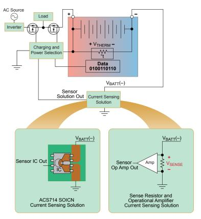
Figure 3. Smart battery current sensing. The Illustration on the left shows the integrated primary sensed current path featured in the ACS714.
