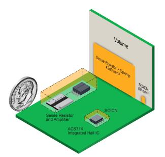
Figure 2. PCB volume comparison of typical Hall current sensor ICs versus traditional sense resistance and operational amplifier current sensing
