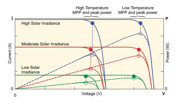
Figure 2. The graph above shows how I-V curves change with both irradiance and temperature. Subsequently, the maximum power point (MPP) will change, and the tracking algorithms must determine the new MPP.
