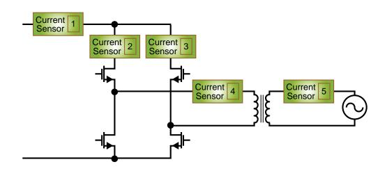
Figure 3. Multiple current sensors are seen in this diagram of a typical inverter configuration. For simplicity, filter components are not shown; however, they will usually be placed on either side of the transformer (if one is used at all), with designers often using the leakage inductance of the transformer as part of the filter.
