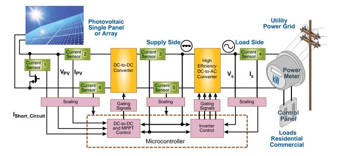
Figure 1. Current sensors are needed throughout grid-tied systems for control of the converters and inverters, optimization of power extraction from solar panels, and fault detection for safety.
