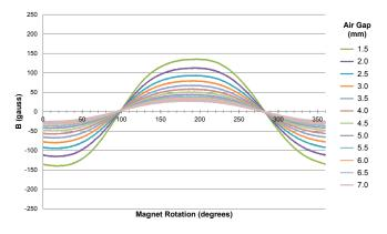
Figure 10: Tangential B-Field Diametral Ring Magnet vs. Air Gap
