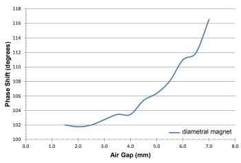
Figure 14: Phase Shift Difference Between Two Falling Edges at the Multipole Ring Magnet Over Air Gap
