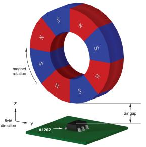
Figure 2: Mechanical Configuration for Case 1
