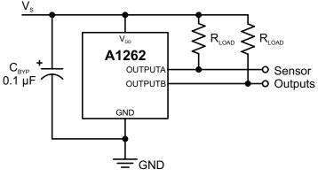
Figure 16: Typical Application Circuit
