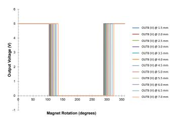
Figure 13: A1262 Multipole Ring Magnet OUTB (tangential) vs. Air Gap As shown in Table 2 below, both outputs also maintain near-ideal ( $\approx$ 50%) duty cycle independent of air gap.
