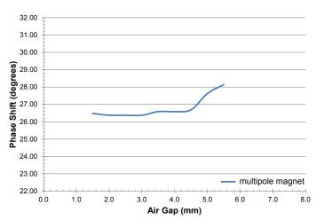
Figure 15: Phase Shift Difference Between Two Falling Edges at the Diametral Magnet Over Air Gap
