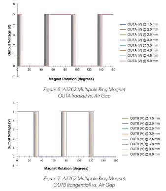
Figure 6 and Figure 7 show the magnetic switching behavior of the two sensor outputs with the 8-pole ring magnet. Given the normal variation in the magnetic switchpoints of the A1262 and a large variation in air gap, the phase relationship of OUTA and OUTB remain very stable. This level of air gap independence is unique to the A1262.
