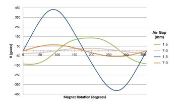
Figure 11: Radial / Tangential B-Field Diametral Ring Magnet vs. Air Gap
