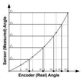
Figure 6: Coordinate transformation into sensor angles
