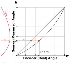
Figure 10: Finding value *X* = *Y* + *C* using the correction curve
