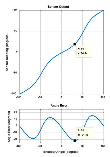
Figure 3: Angle error compared to sensor output plot
