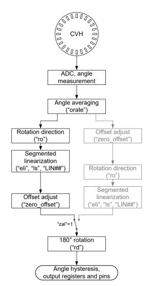
Figure 18: Simplified AAS330x1 signal path with "zal" set to '1'
