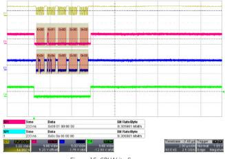
Figure 15: SPI Write Sequence
