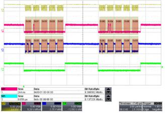
Figure 16: SPI Read Sequence
