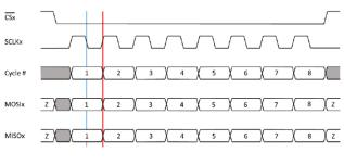
Figure 10: SPI Mode 1, CPOL = 0, CPHA = 1
