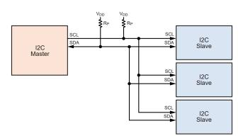
Figure 1: I<sup>2</sup>C bus diagram showing Master and Slave devices
