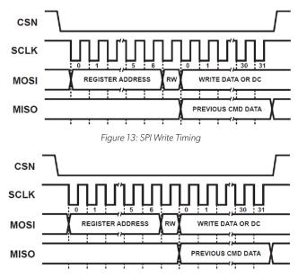
Figure 14: SPI Read Timing
