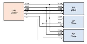
Figure 7: SPI bus diagram showing Master and Slave devices
