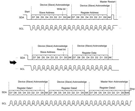
Figure 4: I<sup>2</sup>C Read Timing Diagram
