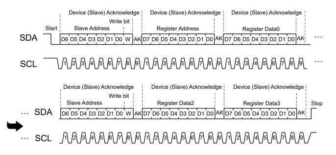
Figure 3: I<sup>2</sup>C Write Timing Diagram
