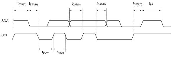
Figure 2: I<sup>2</sup>C Input and Output Timing Diagram
