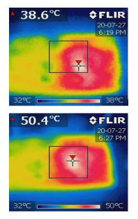
Figure 5: Comparison of steady state temperature increase of the A4480 and a standalone LDO at 12 V, 50 mA current on a 25 mm  $\times$  35 mm PCB.
