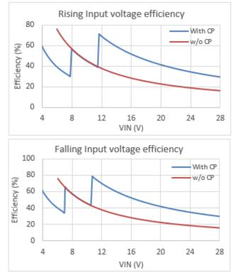
Figure 3: Comparison of steady state efficiencies of the A4480 and an LDO
