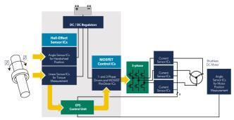
Figure 1: Typical applications of sensors in EPS applications
