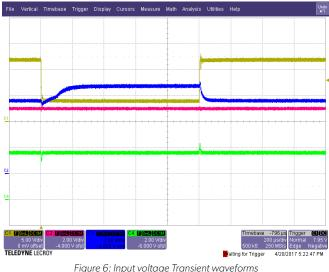
Figure 6: input voltage Transient waveforms C1: VIN, C2: VOUT, C3: VREG, C4: POK
