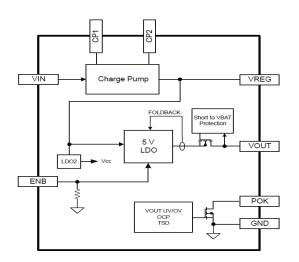
Figure 2: Functional block diagram of the A4480
