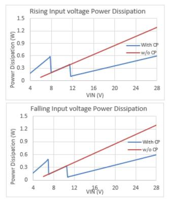
Figure 4: Comparison of steady state power dissipation of the A4480 and a standalone LDO  $\,$
