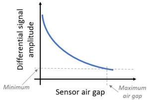
Figure 8: Maximum air gap determination using target mapping
