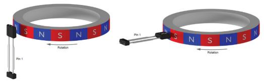
Figure 3: Magnetic field orientation on Allegro Hall based (left only) and GMR (left and right sensor installation) speed sensor
