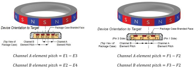
Figure 2: Element pitch representation for GMR (left) and Hall (right) speed and direction sensors
