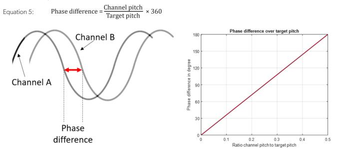
Figure 5: Impact of channel pitch to target pitch ratio on phase difference between differential signals
