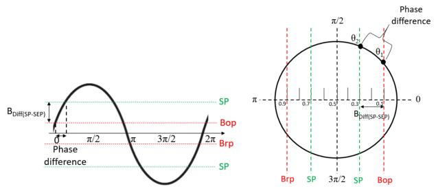
Figure 7: Sine wave (left) and phasor (right) representation of the differential signal. B<sub>OP</sub> (red), B<sub>RP</sub> (red) and SP (green) thresholds respectively represent rising, falling switch point, separation of 20%. In this figure, B<sub>OP</sub> and B<sub>RP</sub> are set to 60% and 40%. Other switch points may be used depending on the sensor of interest and are specified on the datasheet.
