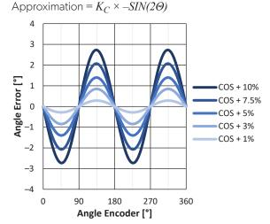
Figure 11: Angle Error from Cosine Amplitude Mismatch
