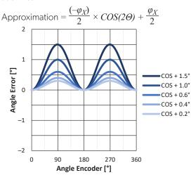
Figure 13: Angle Error from Cosine Phase Error
