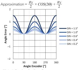
Figure 12: Angle Error from Sine Phase Error
