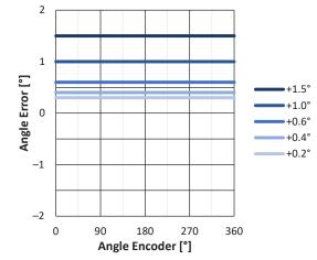
Figure 14: Angle Error from Equal Phase Error
