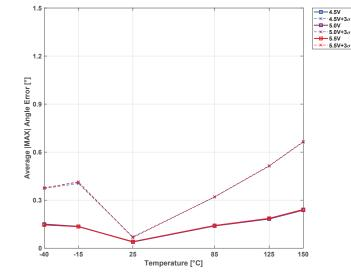
Figure 21: A33230 Average |Max| Dynamic Correction Angle Error +3 $\sigma$  over Temperature and Vcc
