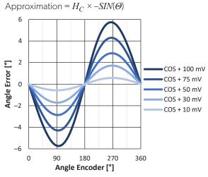
Figure 8: Angle Error from Cosine Offset Error
