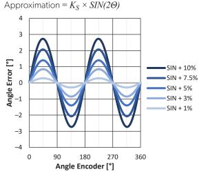
Figure 10: Angle Error from Sine Amplitude Mismatch
