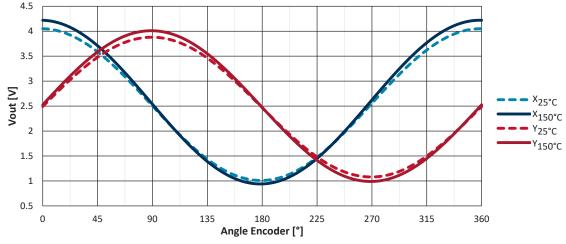
Figure 16: Example OutputA (X), OutputB (Y) Signals at 25°C and 150°C
