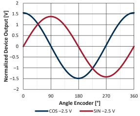
Figure 3: Output with Ideal Offset Removed
