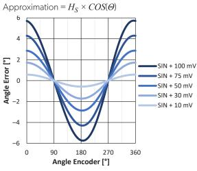
Figure 7: Angle Error from Sine Offset Error
