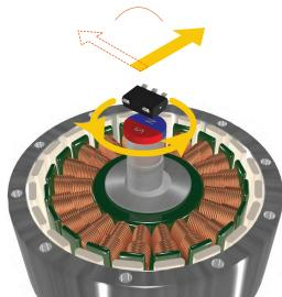
Figure 1: End-of-Shaft Rotary Position Application
