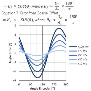
Figure 9: Angle Error from Equal Sine and Cosine Offset Error
