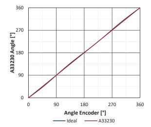
Figure 4: Normalized Device Angle versus Reference Angle
