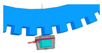
Figure 3: An example image from the simulation software. The steel target is blue and the magnet is turquoise.
