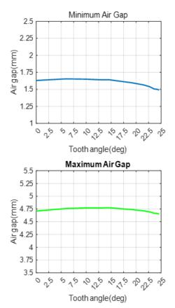
Figure 9: Minimum and maximum air gap as a function of tooth angle with OD = 120 mm, tooth length = 3.1 mm, and valley width = 5 mm.
