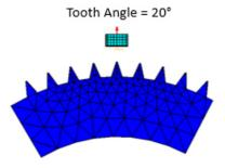
Figure 6: Example image of ferromagnetic target (blue) meshed for simulation with a tooth angle of  $20^\circ$  while retaining root valley width shown in Figure 8.
