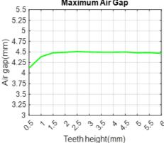
Figure 11: Minimum and maximum air gap as a function of tooth height with OD = 120 mm and tooth length and valley widths = 3.1 mm.
