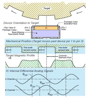
Figure 2: Definition of ATS19580 sensor IC channels.
