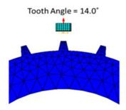
Figure 8: Example image of ferromagnetic target (blue) meshed for simulation with a tooth angle of  $14^\circ$  .
