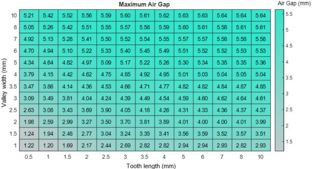
Figure 4: Minimum and maximum air gap as a function of tooth length and valley width for Allegro back-biased sensor IC for a target with an outer diameter of 120 mm.
