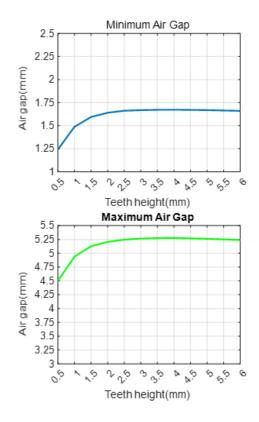
Figure 12: Minimum and maximum air gap as a function of tooth height with OD = 120 mm and tooth length = 3.1 mm and valley width = 5 mm.
