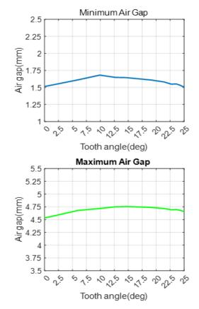
Figure 7: Minimum and maximum air gap as a function of tooth angle starting from the nominal condition (OD = 120 mm, 3.1 mm tooth, 3.1 mm valley, 3 mm tooth height) and decreasing the circular tooth length to increase the tooth angle.
