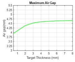
Figure 14: Minimum and maximum air gap as a function of target thickness with OD = 120 mm and tooth length = 3.1 mm and valley width = 3.1 mm.
