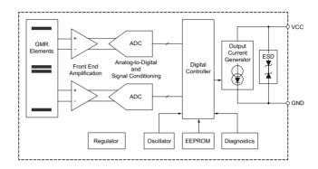
accurate response to low-level differential magnetic signals for reduced controller codes, and prevents flatline conditions in the presence of system perturbations such as thermal gradients, vibration, and air gap dynamics. The differential sensing offers inherent rejection of interfering common-mode magnetic fields.
