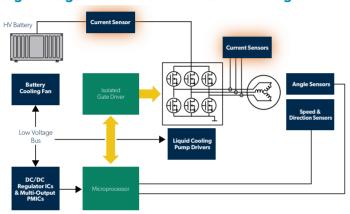
A block diagram for a high voltage traction motor inverter, a common application for the ACS37601, is shown to the left. The current sensors within the diagram are seen highlighted in orange, indicating where the ACS37601 is utilized in the inverter.
