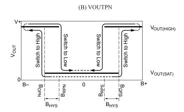
Figure 1. Switching Behavior of Omnipolar Switches. On the horizontal axis, the B+ direction indicates increasing south polarity magnetic field strength, and the B- direction indicates decreasing south polarity field strength (including the case of increasing north polarity). This output switching profile applies when the SELECT line is allowed to float, selecting omnipolar operation.
