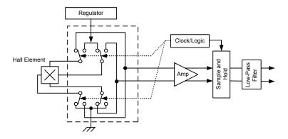
Figure 4. Chopper Stabilization Circuit (Dynamic Quadrature Offset Cancellation)
