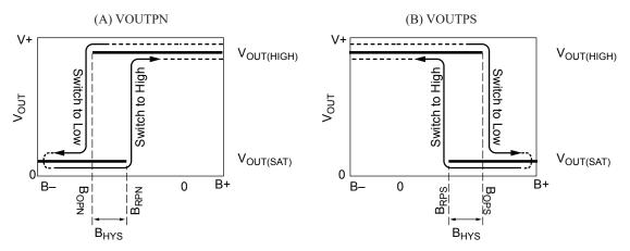
Figure 2. Operation with Unipolar Mode Selected (SELECT Pin Grounded)
