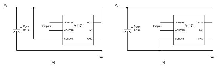
Figure 3. Typical Application Circuits: (a) Omnipolar operation, and (b) Unipolar Operation
