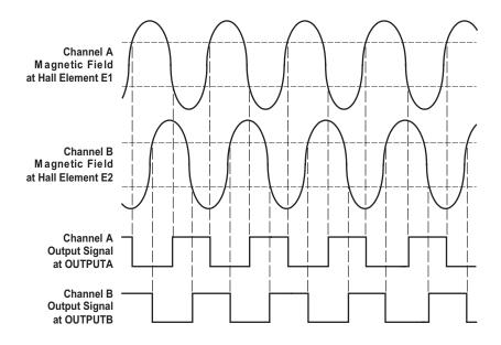
Figure 3: Quadrature Output Signal Configuration.
