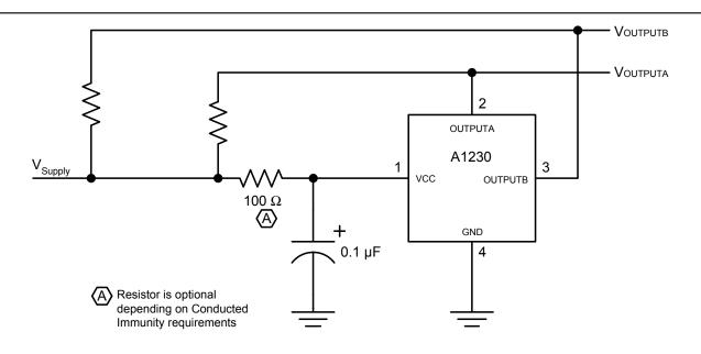
Typical Application using Regulated Supply
