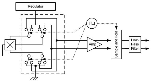
Figure 1: Chopper Stabilization Circuit (Dynamic Quadrature Offset Cancellation)
