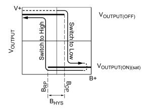
Figure 2: Output Voltage in Relation to Magnetic Flux Density Received.
