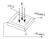
Figure 1: Hall Element, Basic Circuit Operation
