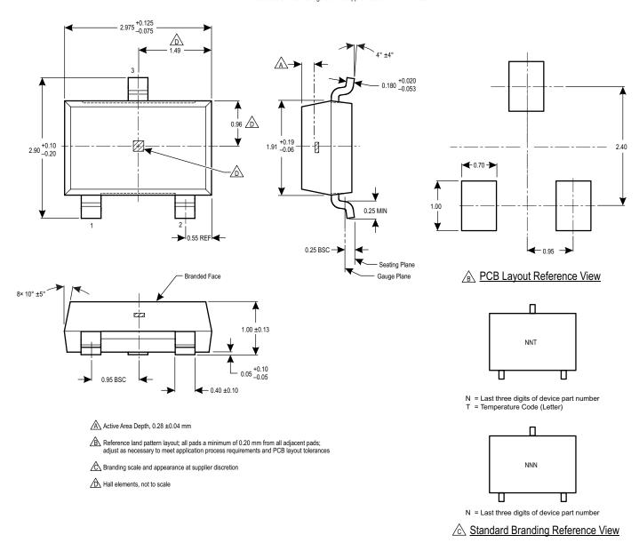
Figure 5: Package LH, 3-Pin SOT23W
