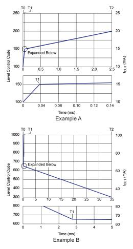
Figure 1. Examples of programmed I<sub>OUT</sub> change
