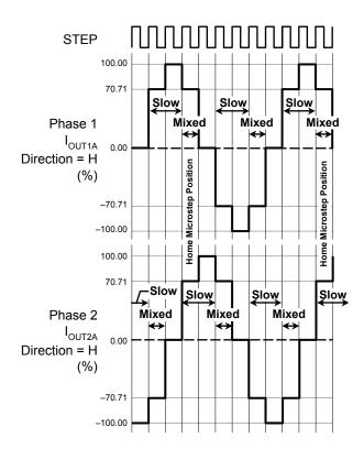
Figure 2. Decay Mode for Full-Step Increments
