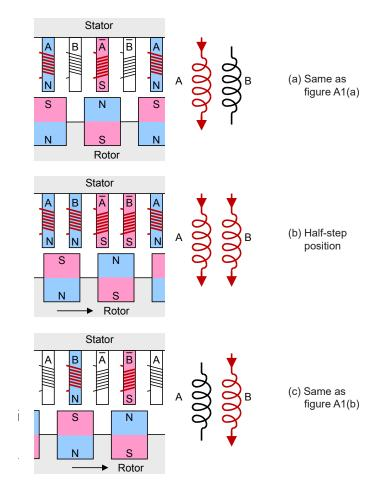
Figure A2. Half step operation
