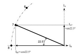
Figure A7. Calculating phase current magnitudes
