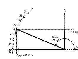
values shown Figure 4. Calculation of resultant motor current
