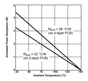
Figure 15. Allowable power dissipation, on typical PCBs
