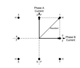
Figure A4. Phase diagram for simple half step
