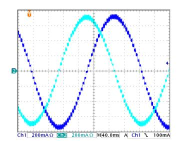
Figure A9. Measured sixteenth-step phase current sequence
