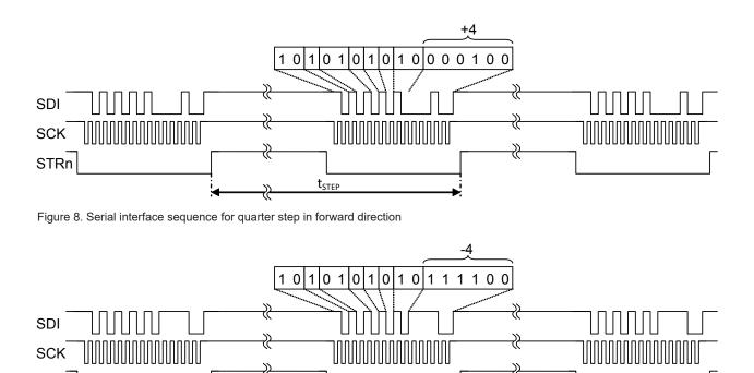
Figure 9. Serial interface sequence for quarter step in reverse direction
