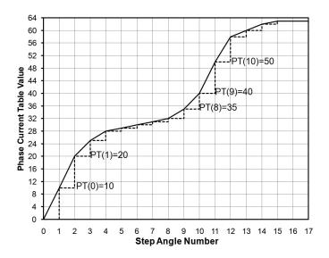
Figure 12. Digitizing the example current profile
