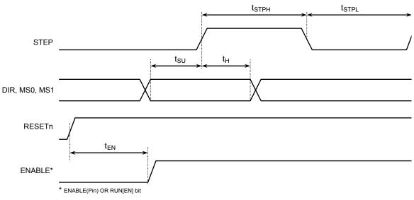
Figure 2. Control Input Interface Timing Diagram
