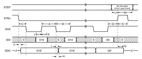
Figure 1. Serial Interface Timing Diagram
