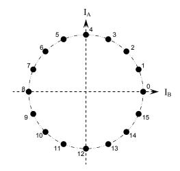
Figure A6. Phase diagram for quarter step
