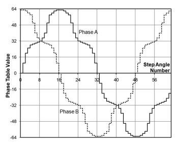
Figure 13. Resulting example current profile
