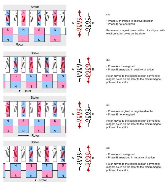
Figure A1. Basic principle of bipolar stepper motor operation
