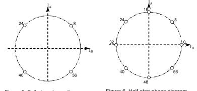
Figure 5. Full-step phase diagram using STEP input
