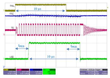
Figure 16: Zoom in view for PWM on-time = 10  $\mu$ s. Notice that the LED current is shifted with respect to PWM signal. Ripple at V<sub>OUT</sub> is ~0.2 V when using 2 × 4.7  $\mu$ F MLCC as output capacitors.
