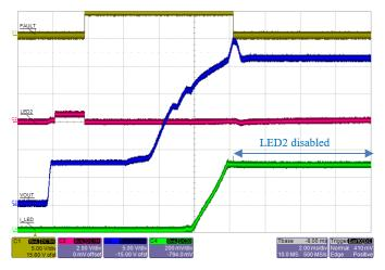
Figure 35: A80602 startup with LED2 string open.  $V_{OUT}$  hits OVP at ~30 V and LED2 is removed from regulation. FAULT pin goes Low but remaining LED strings continue to operate.
