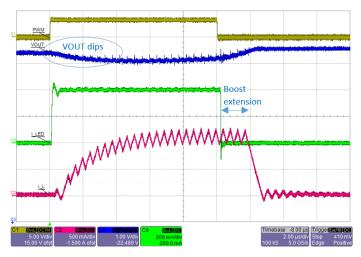
Figure 18: Traditional PWM Dimming operation where boost switch and LED current are enabled at the same time. Note that  $\rm V_{OUT}$  shows overall ripple of ~0.5 V
