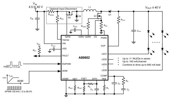
Figure 1: A80602 Simplified Circuit Configuration
