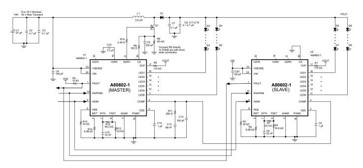
Figure 49: Two A80602-1s connected in master/slave configuration to drive 12 strings of LEDs.
