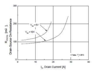
Figure 51: Chart showing On-Resistance varies with Drain Current and Gate Voltage.
