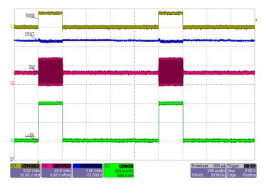
Figure 15: PWM dimming operation at 20% 1 kHz. CH1 = PWM (5 V/ div), CH2 = SW (20 V/div), CH3 =  $V_{OUT}$ , CH4 =  $i_{LED}$  (200 mA/div).
