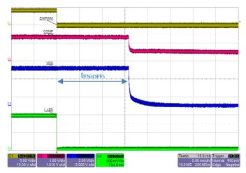
Figure 29: After EN/PWM (Yellow) goes Low for ~16 ms, the IC completely shuts down so both VDD (Blue) and COMP (Red) decay.
