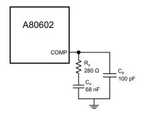
Figure 45: Compensation Network Schematic
