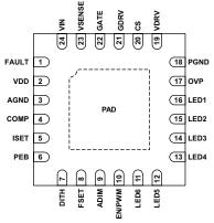
Package ES, 24-Pin QFN Pinouts
