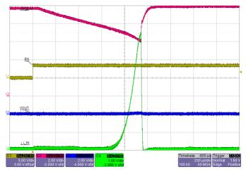
Figure 43: Startup into an output shorted-to-GND fault. Input OCP is tripped when current (Green trace) exceeds ~6.5 A. PMOS Gate (Red) is turned off immediately and IC latches off.
