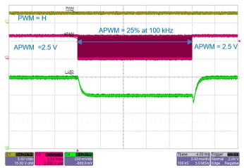
Figure 23: PWM = H. Total LED current drops from 400 mA (4  $\times$  100 mA/ch) to 300 mA when APWM of 25% duty cycle is applied. Note that LED current takes ~1 ms to settle after change in APWM.
