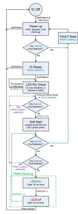
Figure 31: Simplified startup flow chart for A80602-1, showing responses to both Internal and External FAULT signals
