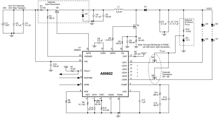
Figure 48: Cascode-Protected LED Pins Design.
