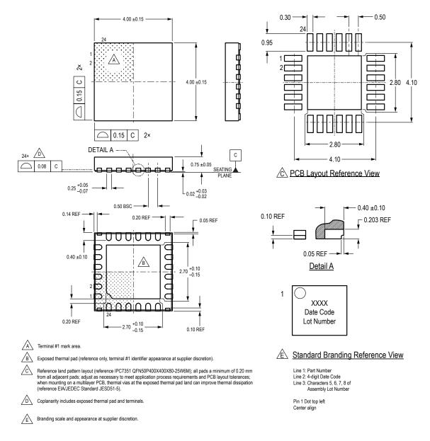
Figure 44: Package ES, 24-Pin 4 mm × 4 mm QFN with Exposed Thermal Pad and Wettable Flank
