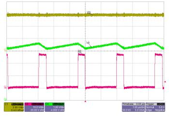
Figure 40: Normal 400 kHz switching waveform at  $V_{\rm IN}$  = 6 V. Red trace is the SW node voltage at 10 V/div. Green trace is the inductor current at 1 A/div.
