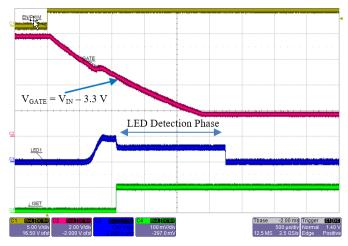
Figure 4: Startup showing EN/PWM, GATE, LED1, and ISET. Note that LED Detection Phase starts as soon as GATE pin is pulled down to 3.3 V below  $V_{\rm IN}$ .
