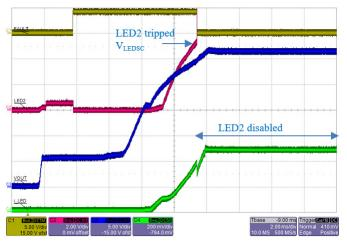
Figure 33: A80602 startup sequence when LED string#2 has a partialshort fault (6 × WLED instead of 8). As soon as LED2 pin rises above  $V_{LEDSC}$  (~5 V), the channel is disabled and FAULT = Low.
