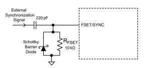
Figure 13: Countermeasure for External Sync Stuck-at-Low Fault
