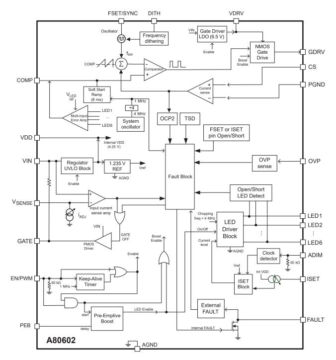
Figure 2: Functional Block Diagram
