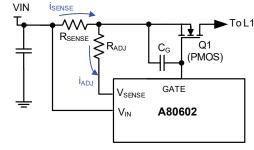
$V_{IN} - V_{SENSE} = R_{SENSE} \times i_{SENSE} + R_{ADJ} \times i_{ADJ}$
