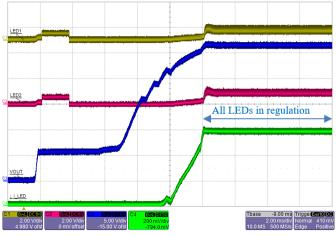
Figure 32: A80602 Normal startup sequence showing voltage at LED1 and LED2 pins.  $V_{IN}$  = 6 V, output = 8 × WLED in series, current = 6 × 100 mA
