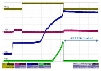
Figure 36: A80602-1 startup with LED2 string open. V<sub>OUT</sub> hits OVP and all LED string are disabled. FAULT pin goes Low and IC remains latched off until reset.
