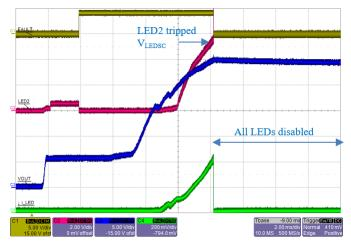
Figure 34: A80602-1 startup sequence when LED string#2 has a partial-short fault (6 × WLED instead of 8). As soon as LED2 pin rises above  $V_{LEDSD}$  (~5 V), the channel is disabled but FAULT remains High.
