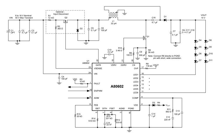
Figure 47: SEPIC configuration. Allows operation with  $V_{IN}$  both above and below  $V_{OUT}$ .
