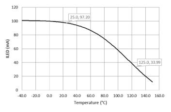
Figure 28: LED current varies with temperature when using thermistor NTCS0805E3684JXT for thermal foldback
