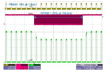
Figure 24: PWM = 10% at 1 kHz. Peak LED current drops from 400 mA (4 × 100 mA/ch) to 300 mA when APWM of 25% duty cycle is applied
