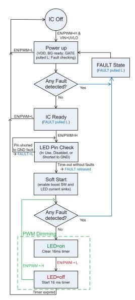
Figure 30: Simplified A80602 Startup Flowchart
