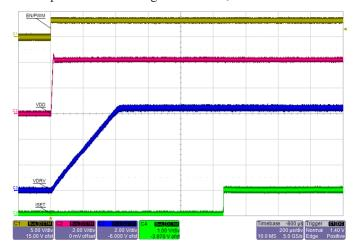
Figure 3: Startup showing (from top to bottom) EN/PWM, VDD, VDRV, and ISET.
