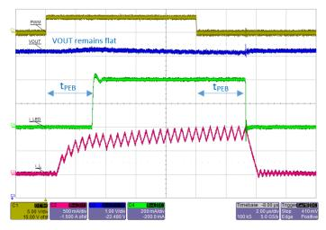
Figure 19: A80602 PWM dimming operation with PEB delay set to 3  $\mu s.$  Note that  $V_{OUT}$  ripple is reduced to ~0.2 V.
