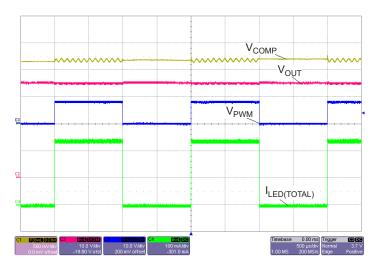
Figure 8: Typical PWM Diagram Showing V<sub>OUT</sub>, I<sub>LED</sub>, and COMP Pins, as well as the PWM Signal. (PWM dimming Frequency is 500 Hz 50% duty cycle.)
