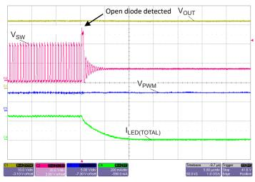
Figure 23: Open Schottky Diode Protection
