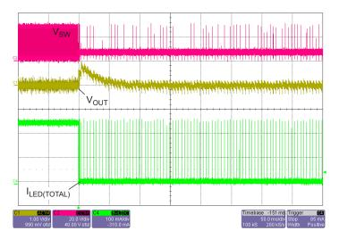
From PWM = 100% to PWM = 0.01% at 120 mA/Channel,  $V_{\rm IN}$  = 12 V; Time base = 50 ms/Div
