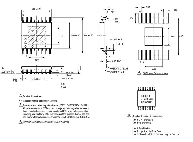
Package LP, 16-Pin TSSOP with Exposed Thermal Pad
