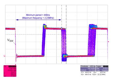
Figure 32: Maximum Dithering Switching Frequency = 2.23 MHz at V<sub>IN</sub> = 12 V, and PWM Ratio = 100%
