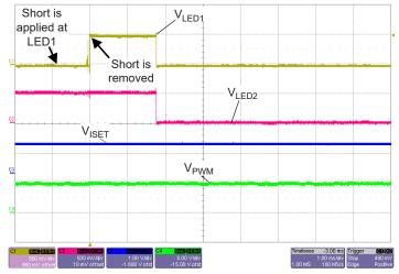
Figure 6: One LED is Shorted to GND. The IC will not proceed with power up until LED pin is released, at
