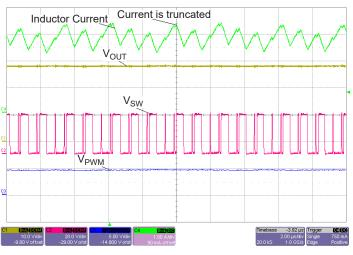
Figure 25: Cycle-by-Cycle Current Limit
