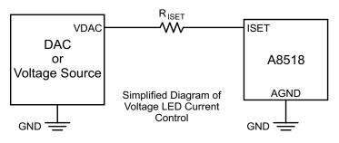
Figure 18: Typical Application Circuit Using a DAC to Control the LED Current in the A8518
