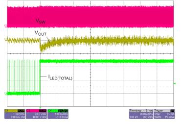
From PWM = 0.1% to PWM = 100% at 120 mA/Channel,  $V_{IN}$  = 12 V;
