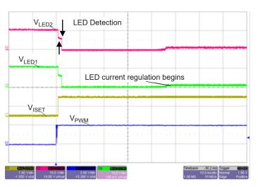
Figure 4: LED String Detect Occurs when Both LEDs are Selected to be Used
