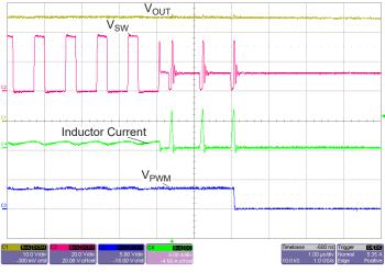
Figure 26: Secondary Boost Switch OCP
