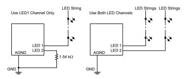
Figure 3: Channel Select Setup
