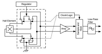
Figure 5: Concept of Chopper Stabilization Technique
