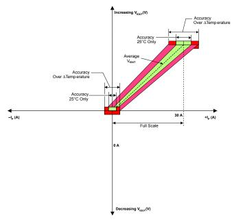
Figure 1: Output Voltage versus Sampled Current
