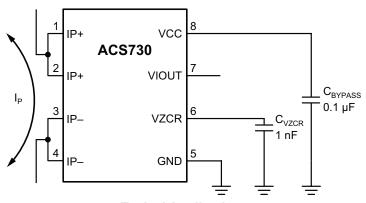
The ACS730 outputs an analog signal, V<sub>IOUT</sub>, that varies linearly with the bidirectional AC or DC primary sensed current, I<sub>P</sub>, within the range specified.
