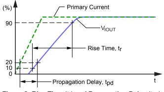
Figure 8: Rise Time (t<sub>r</sub>) and Propagation Delay (t<sub>nd</sub>)
