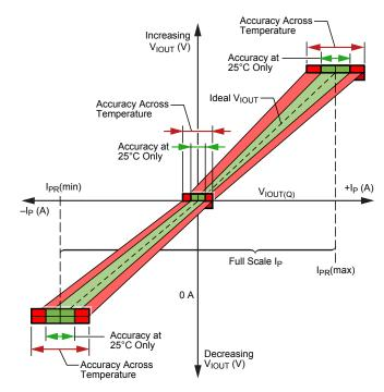
Figure 1: Output Voltage versus Sensed Current
