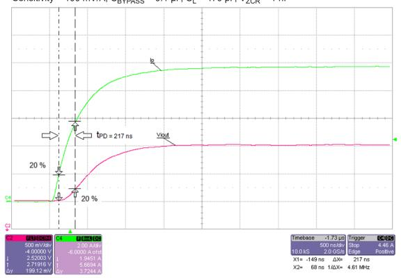
Rise Time (t<sub>r</sub>) 10 A input signal (I<sub>P</sub>) with rise time < 1  $\mu$ s Sensitivity = 100 mV/A, C<sub>BYPASS</sub> = 0.1  $\mu$ F, C<sub>L</sub> = 470 pF, V<sub>ZCR</sub> = 1 nF
