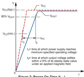
Figure 7: Power-On Time (t<sub>PO</sub>)
