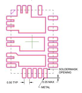
Figure 20: Recommended PCB Footprint
