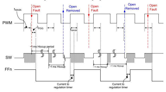
Figure 11b: LED Open Fault Timing Diagram Overview
