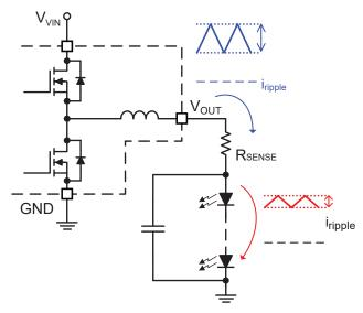
With a small capacitor across LED string: Ripple current through LED string is reduced, while ripple voltage across Rsense remains high.
