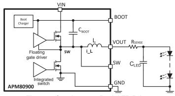
Figure 4: Synchronous Buck LED Driver
