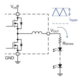
Without output capacitor: The same inductor ripple current flows through sense resistor and LED string.
