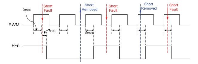
Figure 11a: LED Short Fault Timing Diagram Overview
