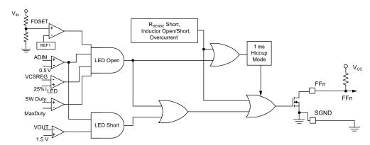
Figure 9: LED Open/Short Fault Block Diagram
