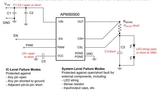
Figure 12: Demonstration of various possible fault cases in an application circuit
