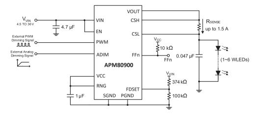
Figure 1: APM80900 Typical Application Circuit
