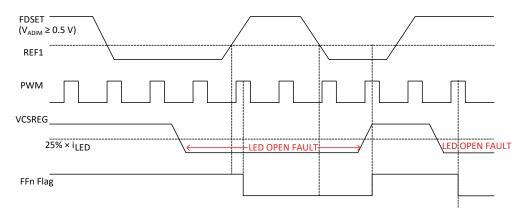
Figure 10: LED Open/Short Fault Timing Diagram
