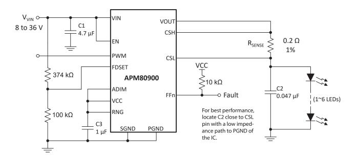
Figure 14: Application circuit example for APM80900 with 1 A LED current.
