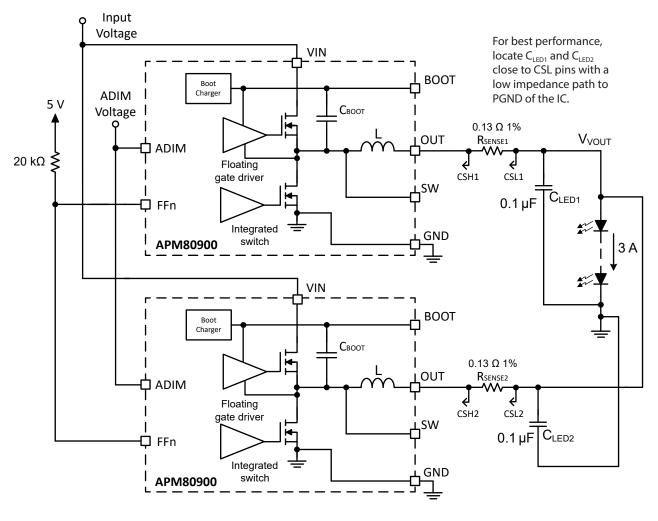
Figure 16: Using 2 (or more) APM80900s in parallel to drive the same LED string.
