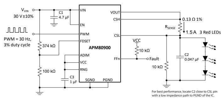
Figure 18: Application circuit example at  $V_{VIN}$  = 30 V ±10% to drive 3 red LEDs @ 1.5 A with external PWM dimming at 30 Hz, 3% duty cycle.
