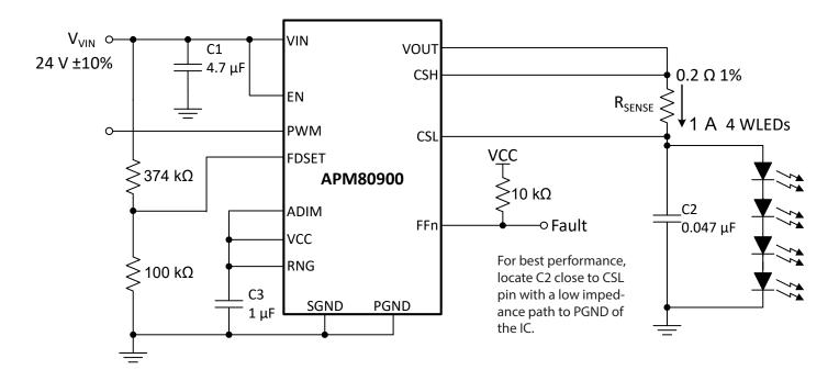
Figure 15: Application circuit example with  $V_{VIN}$  = 24 V ±10%, 4 WLEDs @ 1 A
