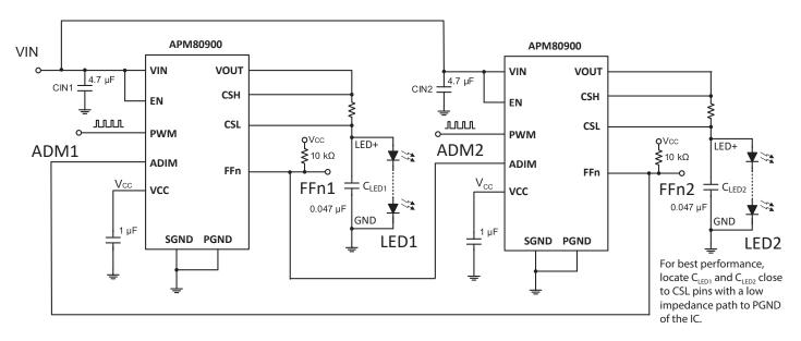
Figure 17: "One Out All Out" functionality can be implemented with 2 APM80900s driving different LED strings:
