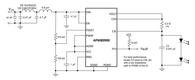
Figure 3: EMC test circuit
