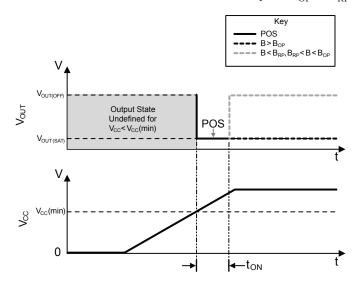
Figure 2: Power-On Sequence and Timing
