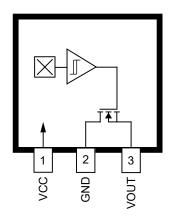
LH Package, 3-Pin SOT23W Pinout
