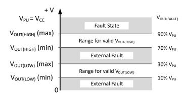
Figure 6: APS12450 valid (typical) and fault-condition output levels
