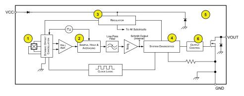
Figure 3: Diagnostics Coverage Block Diagram
