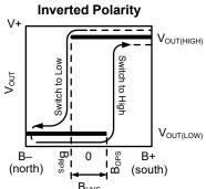
Figure 1: Hall latch magnetic and output polarity options B- indicates increasing north-polarity magnetic-field strength, and B+ indicates increasing south-polarity magnetic-field strength.
