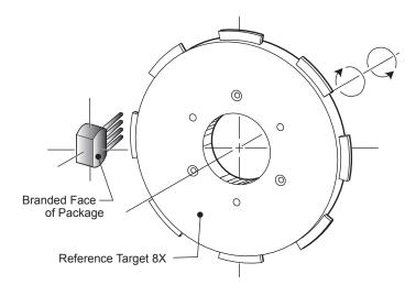
Figure 4. Configuration with Reference Target
