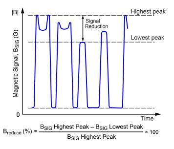
Figure 3. Definition of Maximum Allowable Signal Reduction,  $B_{reduce}$ , as a percentage of the overall magnetic signal.
