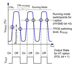
Figure 7. Calibration mode waveforms.
