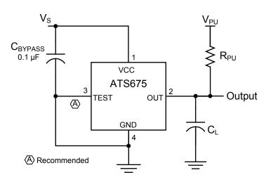
Figure 1. Operational circuit for the ATS675
