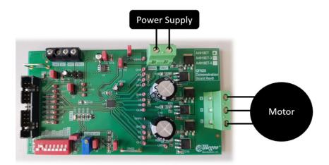
Figure 2: Connection diagram for motor and supply connections
