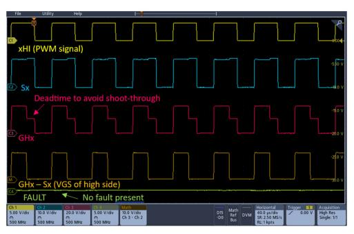
Figure 3a: Correct operation showing the high-side driver
