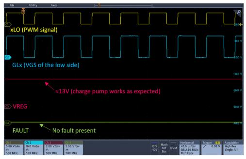
Figure 3b: Correct operation showing the low-side driver
